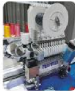
◎ 简易绳绣 Easy cording device
